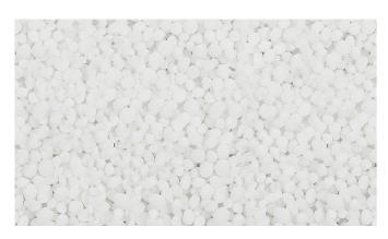
Appearancewhite granularMax. Solubility1,200 g/l at 20 °CElectrical Conductivity1.25 mS/cmBulk density1.1 kg/lpH-value in 10 % solution5.7 - 7.0Chloride as Cl< 0.1 %</th>
