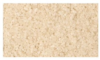
**Appearance** White crystals 750 g/l at 20 °C Max. solubility **Electrical conductivity** 65.2 mS/cm (1% solution) **Bulk density** 950-1100 kg/m<sup>3</sup> pH-value in 10% solution 4-5 Insoluble (H<sub>2</sub>O) ≤0.1%
